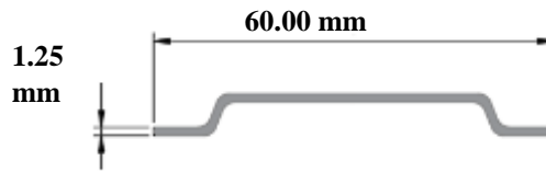
Figure 06: Dimensions and shape of the fiber used.
