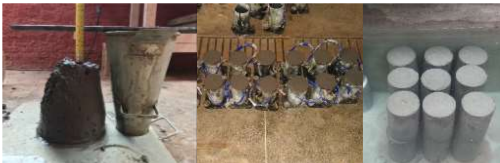
Figure 05: Molding and curing of the elements.
