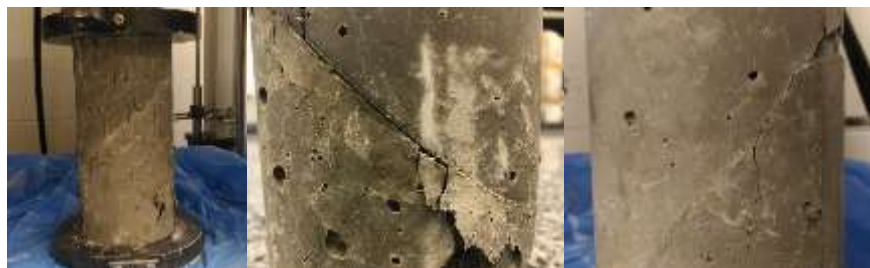
Figure 19:CJDS rupture compression test
