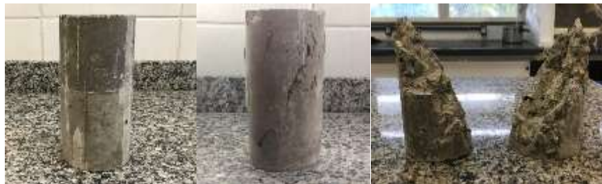
Figure 18:CJHS rupture compression test
